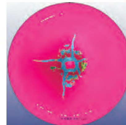
(a) ASU model prediction showing damage and localized failure
