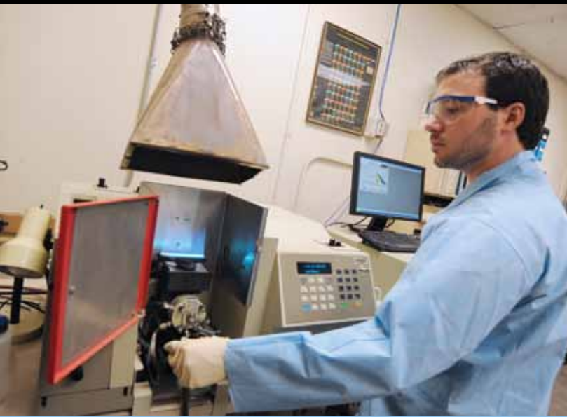
An atomic Absorption Spectrophotometer is used to measure metal concentrations in water.
