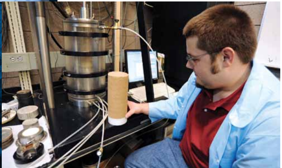
Soil-Water Characteristic Curve Testing in the Unsaturated Soil Mechanics Laboratory
