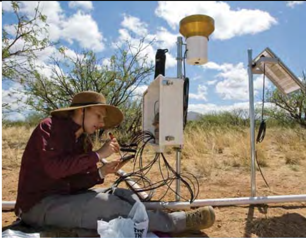
SSEBE Graduate student Nolie Pierini installs wiring for soil moisture and temperature sensors and a rain gauge at the Santa Rita Experimental Range near Green Valley, Arizona (Photo: Tom Story)
